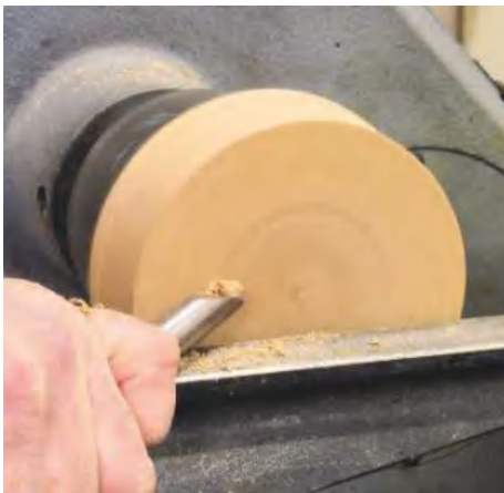
▲ Pic.4 Now the hole is drilled you're ready to start turning. The base is held on a screw chuck. True up the bottom with a pull cut or use a scraper to remove any ridges left by the gouge
